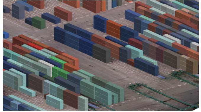
Fig. 14. Subset of the 3-D reconstructed container terminal. Each container is a tangible 3-D object featuring positional, colorimetric, geometric, and identification attributes. Stacked containers were visualized in the same color of the container on top, according to the per-object mean RGB value extracted from the RGB orthophoto.
