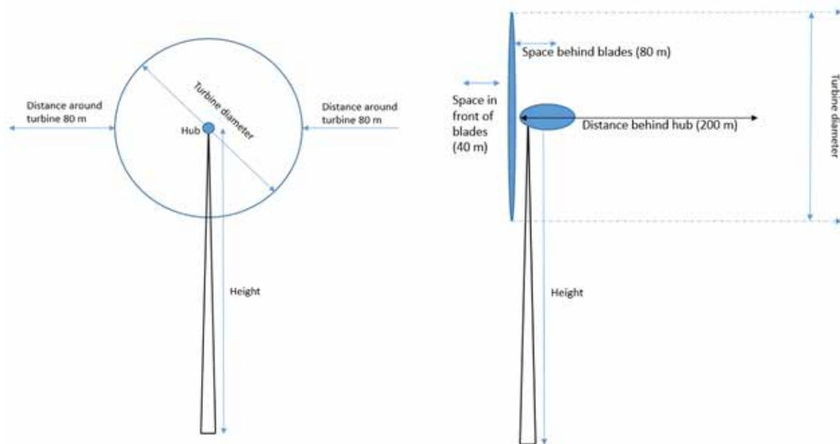
To calculate the clear area needed around each turbine:
