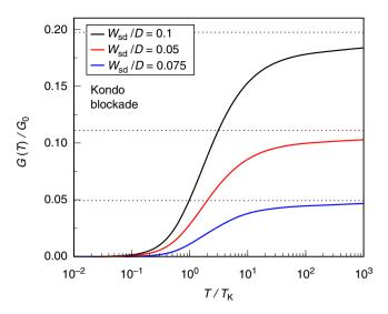
Figure 4 | Kondo blockaded conductance near a quantum interference node in the exchange cotunneling. NRG results for the conductance G(T) as a function of rescaled temperature  $T/T_{\rm K}$  at  $J_{\rm sd}=0$  for various  $W_{\rm sd}$ , showing in all cases an overall conductance node G(0)=0. Plotted for  $J_{\rm ss}=0.25D$ ,  $J_{\rm dd}=0.2D$  and  $W_{\rm ss}=W_{\rm dd}=0$ . Dotted lines show the high-temperature perturbative expectation.
