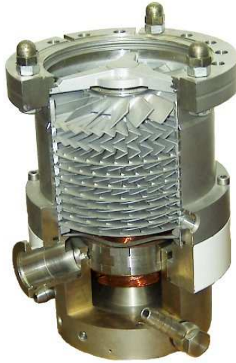
Figure 1.10: Cut-away turbo-molecular pump
