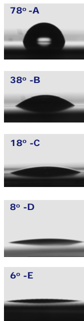
Figure 2: The effect of increasing plasma exposure time on water contact angle
