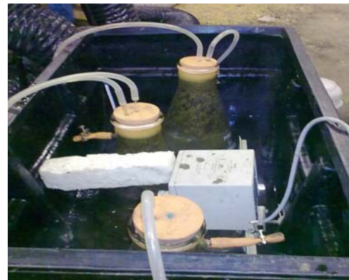
Figure 2: Digesters in water bath with heat pump.
