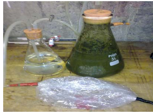
Figure 1: Diagram representing a bench scale anaerobic digester
