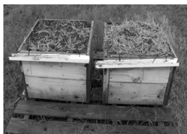
Figure 1: Purpose-built soil boxes (0.6m x 0.6m x 0.45m) with 2 levels of straw incorporation: 3t ha -1 (left) and 10t ha -1 (right)
