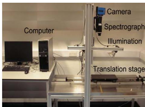
Figure 1. Hyperspectral imaging system used for image acquisition
