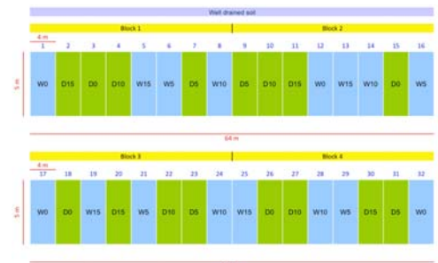
Figure 2. Diagram of a randomised plot layout design with assigned SMD on wetting and drying cycle for the well drained soil type.
