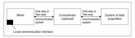
**Figure 2: General structure of a smart metering system** (Source: Figure 6, ERGEG Status Review of Regulatory Aspects of Smart Metering<sup>6</sup>)
