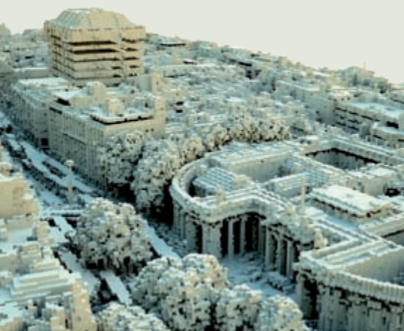
Tommy Hinks' image 'Digital Dublin'. During a flyover of Dublin, a dataset containing 225 million point samples was collected. Through building a recursively subdividing cuboid data-structure, large parts of the dataset can be visualized and understood. Depicted in the image is a small part of the data set covering Dame Street with surroundings. Originally submitted for UCD Images of Research competition.
