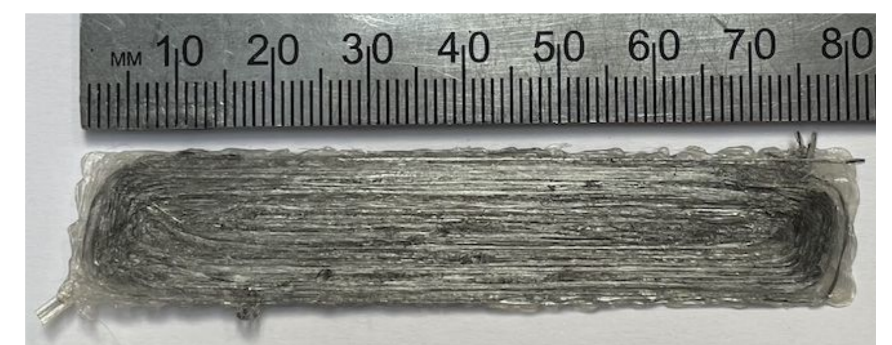
Fig 21. Fused Filament Fabrication of Nylon with SSF
