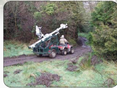
Figure 1. The roving EC tower in situ at the 6 year old Sitka site, at the 11 year old Ash site and in transit between sites
