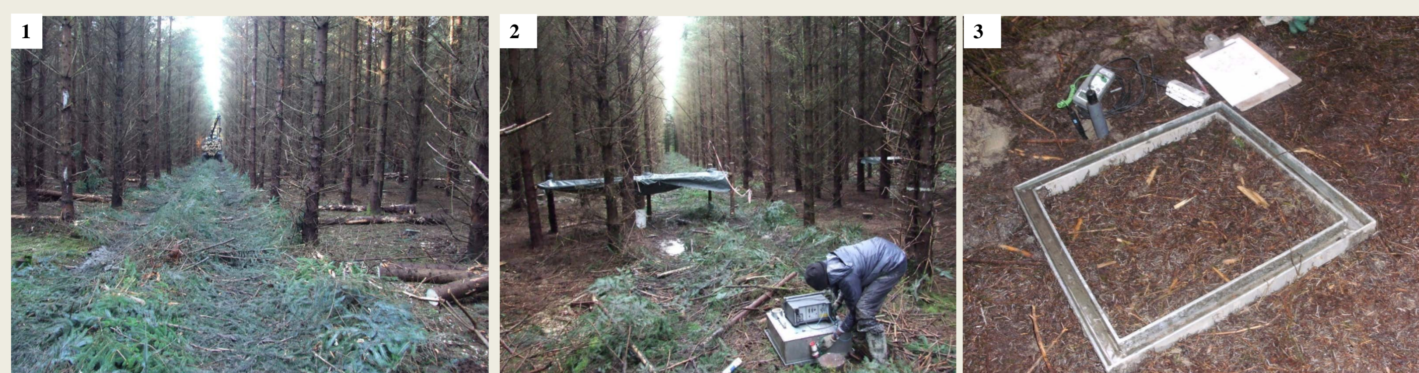
Pictures L - R : (1.) Brush lane used for evacuating felled logs, (2.) Efflux measurements from brush lane, (3.) Collar inserted into forest floor and thetaprobes used for soil moisture measurements.
