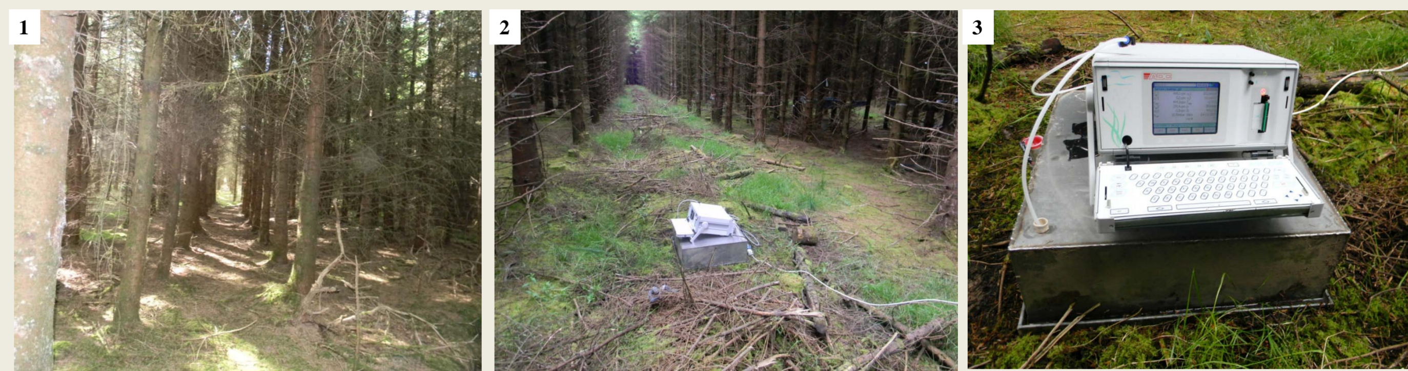
Pictures L - R : (1.) Forest floor, (2.) Efflux measurements' set up (3.) Infra red gas analyser and static chamber.
