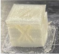
Fig 19. Nylon Calibration Cube
