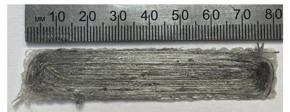
Fig 21. Fused Filament Fabrication of Nylon with SSF
