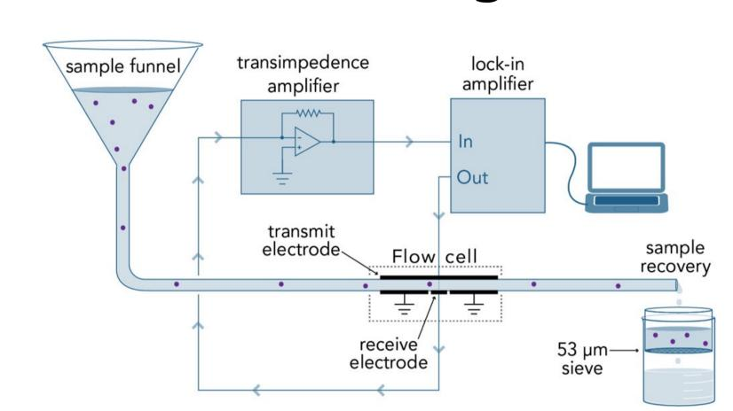
**Fig. 4.** Impedance Spectrometer Design [2]
