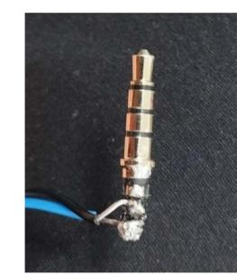
Fig. 1. Top left to bottom right: Aluminum foil was adhered with glue to cardstock, with sample cuvette. A cardboard box was cut into to create a support structure. Circuit diagram. A stripped TRRS audio jack is shown on the right, with two wires soldered on.
