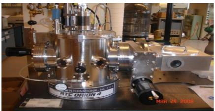
Figure 3: Sputter deposition chamber
