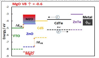
Figure 2: Diagram illustrating band gap of window layers in CdTe solar cell
