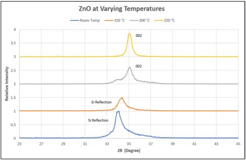
Figure 5: XRD analysis of ZnO at 150 W at various temperatures
