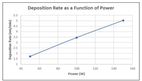
Figure 4: ZnO deposition rate as a function of power at room temperature
