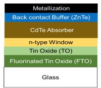
Figure 1: Layers in a CdTe solar cell
