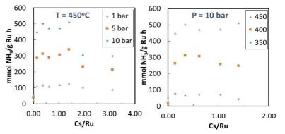
was to determine if the increase in synthesis rate provided by the use of caesium was sufficient to justify the associated increase in cost. The results (shown above) indicated that, for the conditions of temperature and pressure investigated, a significant increase in ammonia synthesis rate could be achieved; most interestingly, optimal results were achieved with a caesium-to-ruthenium ratio of just 0.3, representing a significant cost saving relative to earlier estimates.
