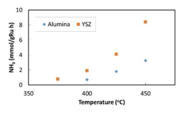
time, to achieve the desired uptake of catalyst (ruthenium oxide). I tested ammonia synthesis rates using both YSZ supports and traditional alumina supports. To the left is a plot comparing rates of ammonia synthesis using these different supports. As anticipated, over the synthesis temperature range investigated, YSZ consistently yielded higher ammonia synthesis rates than alumina.
