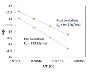
very significant finding, for which there was no prior reference in the literature, for any support. The Wolden-Way group hypothesized that the observed change was due to a change in morphology of the catalyst surface.
