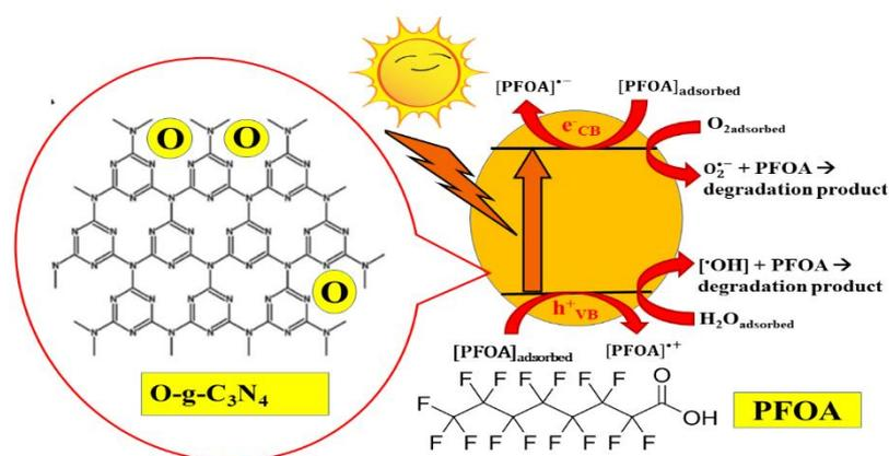
*A cartoon of photocatalytic degradation of PFOA in water using solar light*
