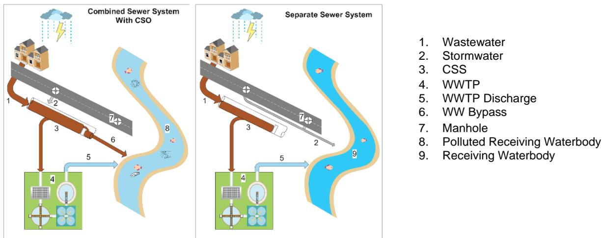
Figure 1: Combined and separate sewer system.
