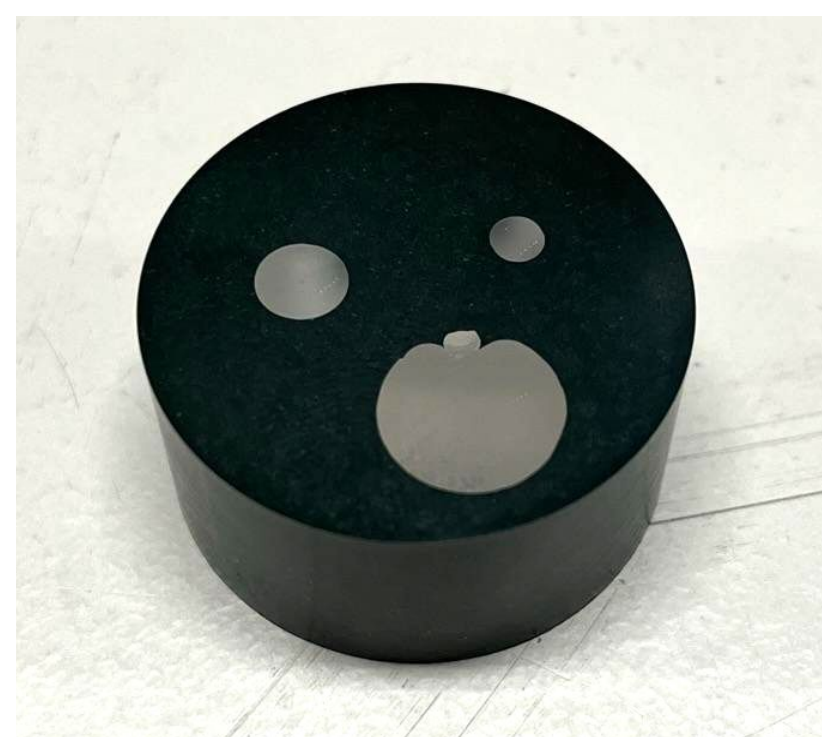
Fig. 2: Mounted and polished heat treated samples
