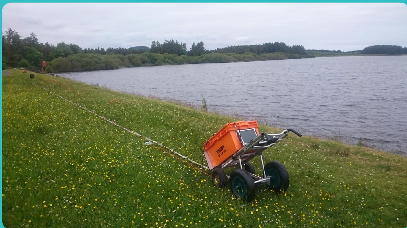
travel through the structure,” he explains. “We found that we could pick up changes in soil moisture and pore pressure, which are related to the stability of the structure, and use that information to build up 2D and 3D images to help identify where a failure could occur.”
