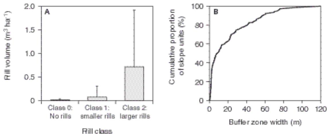
**Figure 4** Measured rill erosion volume in the three classes of rill sizes (RILL class 0, 1 and 2) (A) and width of the buffer zones bordering the investigated slope units (B).
