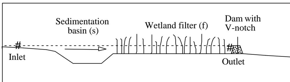
Figure 1. Berg constructed wetland, with composite samplers (#) in the inlet and outlet. Redox electrode was located close to the outlet sampler. The CW covers 0.06 % of the watershed area.
