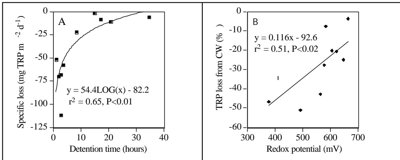
**Figure 3.** Specific loss (A) and relative loss (B) of total reactive phosphorus (TRP) from wetland Berg was correlated to changes in the detention time and redox potential in the CW, respectively.
