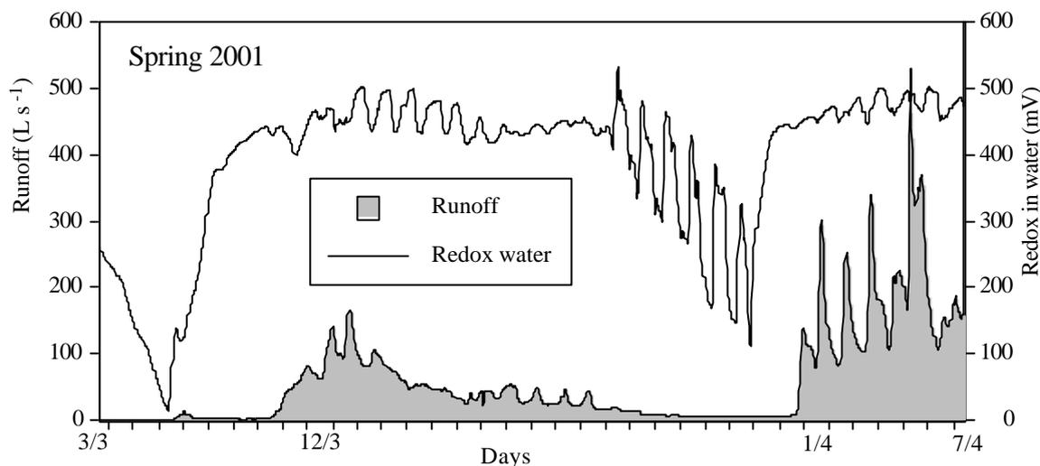
**Figure 4.** Half-hourly observations of runoff and redox potential in Berg CW. The period covers 3 composite sample episodes (start and stop at indicated dates).
