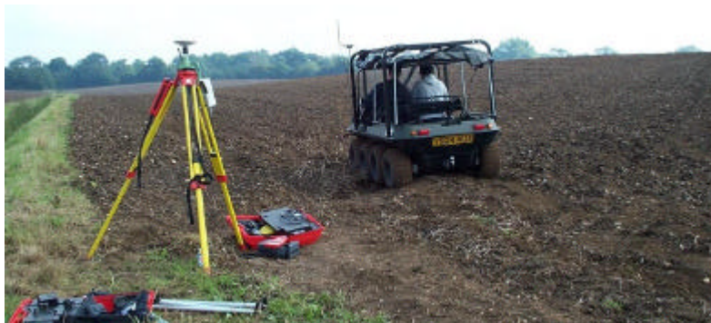
Figure 1, GPS base station and the Green machine about to map a large agricultural field.
