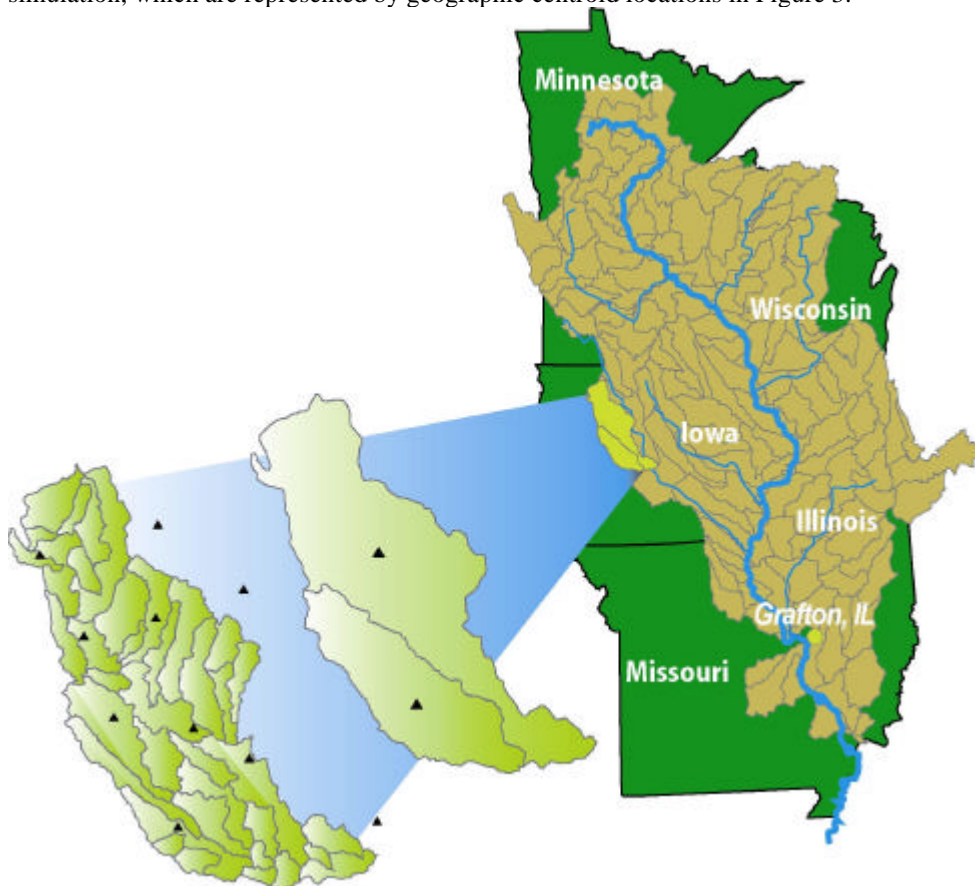
Figure 3. Location of the Raccoon River Watershed in the UMRB, configurations of the 2- and 38-subwatershed simulations, and the locations of the climate stations for the two simulations.
