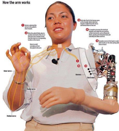
How the arm works
