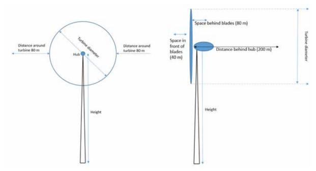
To calculate the clear area needed around each turbine:
