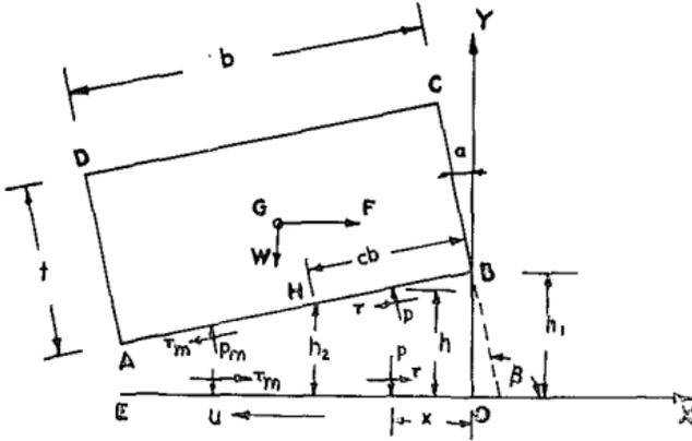
FIG. 2: A cross section of a "boulder" inclined above a plane [3]. An incident water wave would impact from the right. Note changes in notation compared to section II A; boulder height, previously  $a$ , is now  $t$ , and boulder width,  $c$  (as would extend into the page), is now  $w$ . In this case,  $c$  is taken to be  $HB/AB$ , the ratio of the lubricated boulder section to its entire length.
