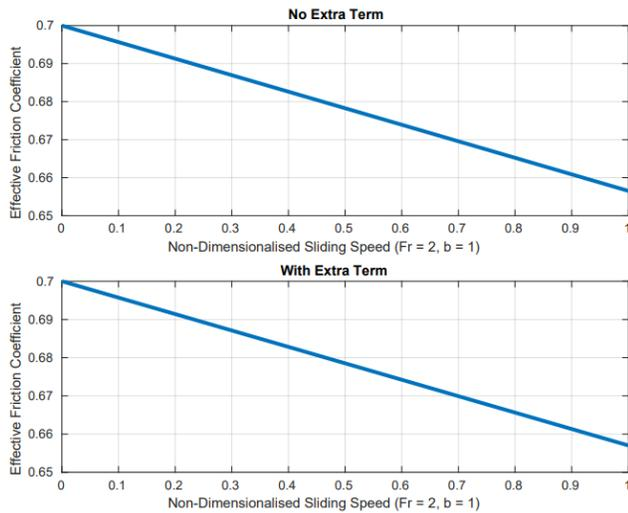
FIG. 5: A comparison of the evolution of  $\mu$  with nondimensionalised sliding speed, with and without the extra shear stress term.
