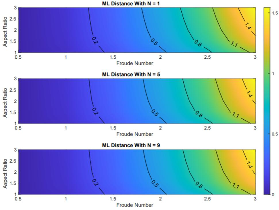
FIG. 8: Nondimensionalised distance moved by the boulder under the mixed-lubrication model for changing  $N$ .
