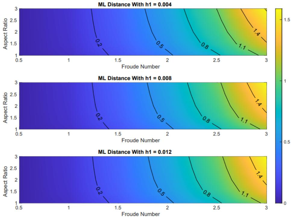
FIG. 7: Nondimensionalised distance moved by the boulder under the mixed-lubrication model for changing  $h_1$ .
