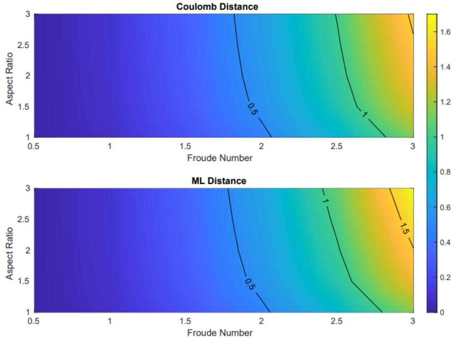
FIG. 6: Nondimensionalised distance moved by the boulder under Coulomb and mixed-lubrication (ML) friction models for various values of Froude number and aspect ratio. Here,  $h_1 = 0.005\text{m}$ .
