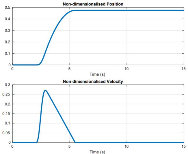
FIG. 3: Evolution of nondimensionalised boulder position and velocity with time.
