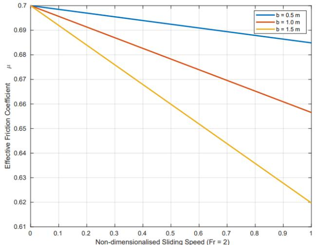
FIG. 4: Evolution of  $\mu$  with sliding speed, for varying values of boulder length  $b$ . Here,  $Fr = 2$ ,  $w = 1\text{m}$ .
