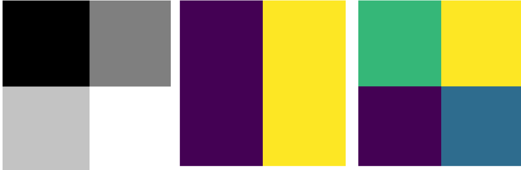
Figure 2: A simple example of a piecewise constant image (left), its two phase segmentation (middle), and its multiphase segmentation (right).
