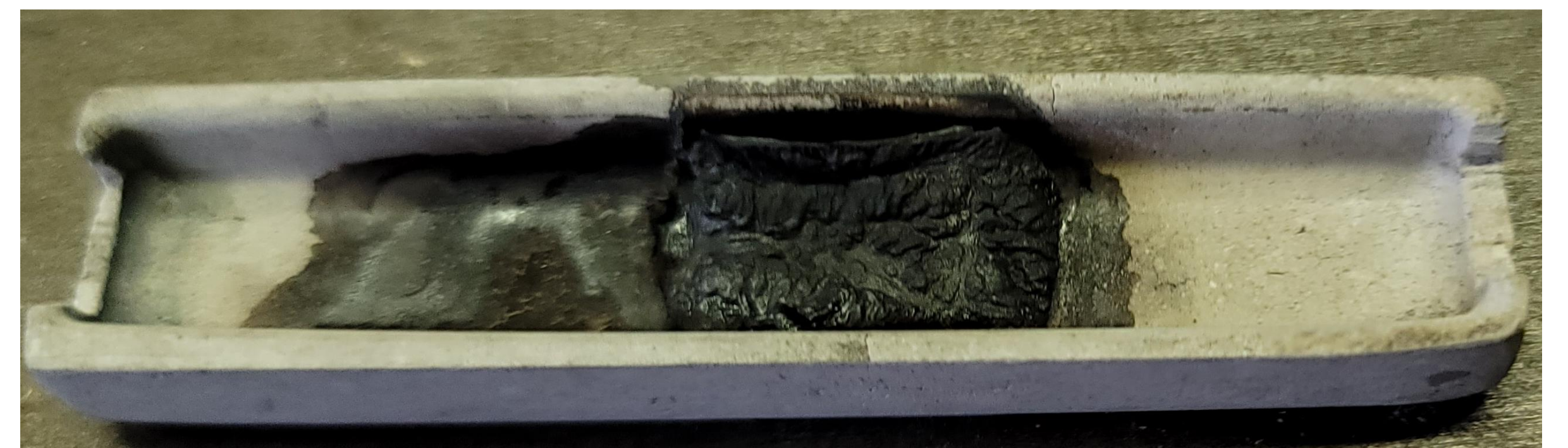
PP sample after heat treatment. A lot of residue was left being possibly indicating the polymer burned instead of vaporizing
