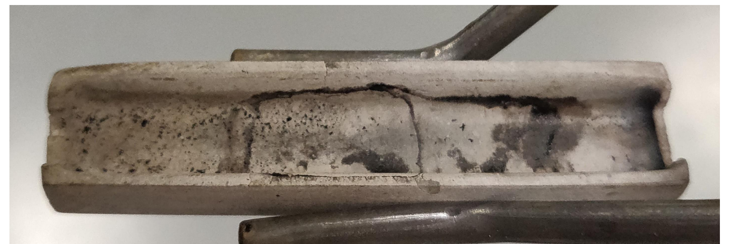
PLA Sample after heat treatment left nearly no residue behind
