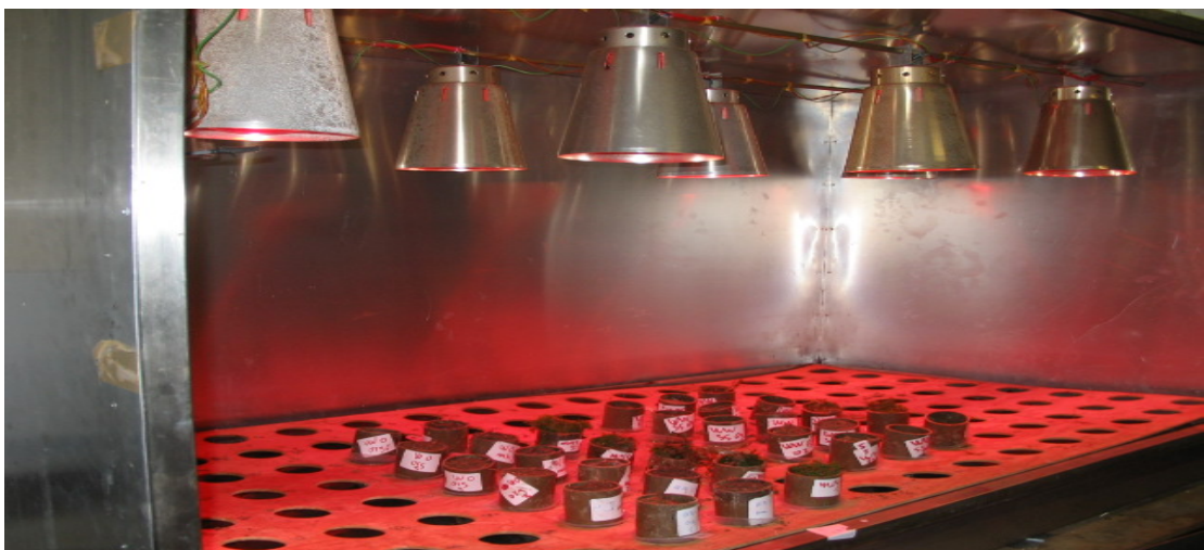
Figure 2.41. The Kempson bowl extractor in use
