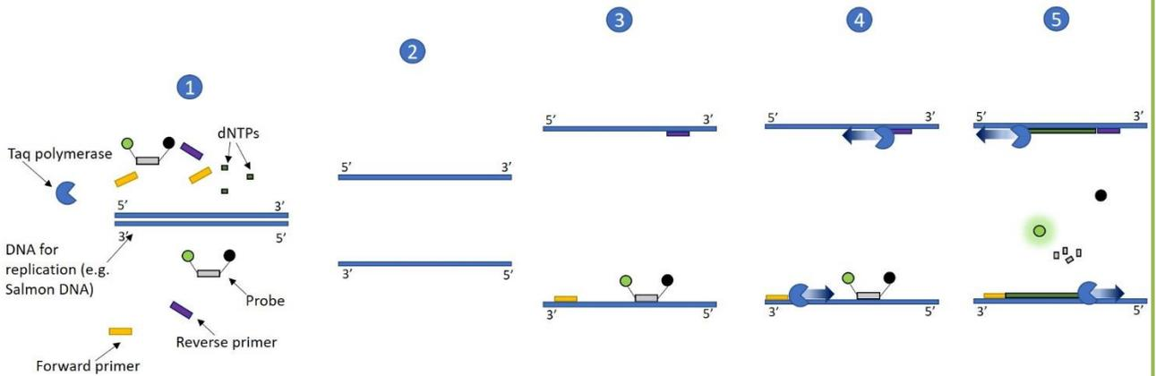
1. Double-stranded DNA for amplification is mixed with qPCR reagents including species specific primers and probe. The probe has a fluorescent reporter dye (pictured in green) and a quencher (black) attached to it. The quencher prevents the reporter dye from fluorescing.
