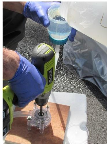
**Fig. 4.** Bernie Ball from the Reconnect project team filtering an eDNA water sample on site using a peristaltic pump powered by a hand drill.
