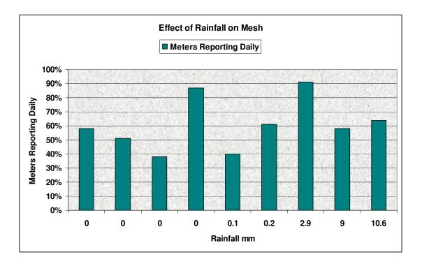
From these measurements we can assume that typical rainfall has no impact on the performance of RF Mesh.
