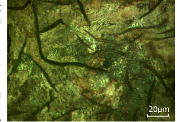
Fig.1: Microstructure of Grey Cast Iron; dark graphite flakes in a predominantly pearlitic matrix
