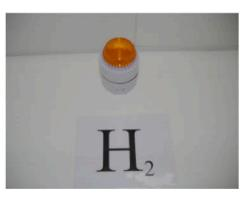
Figure 2. Hydrogen Detection Amber Strobe
