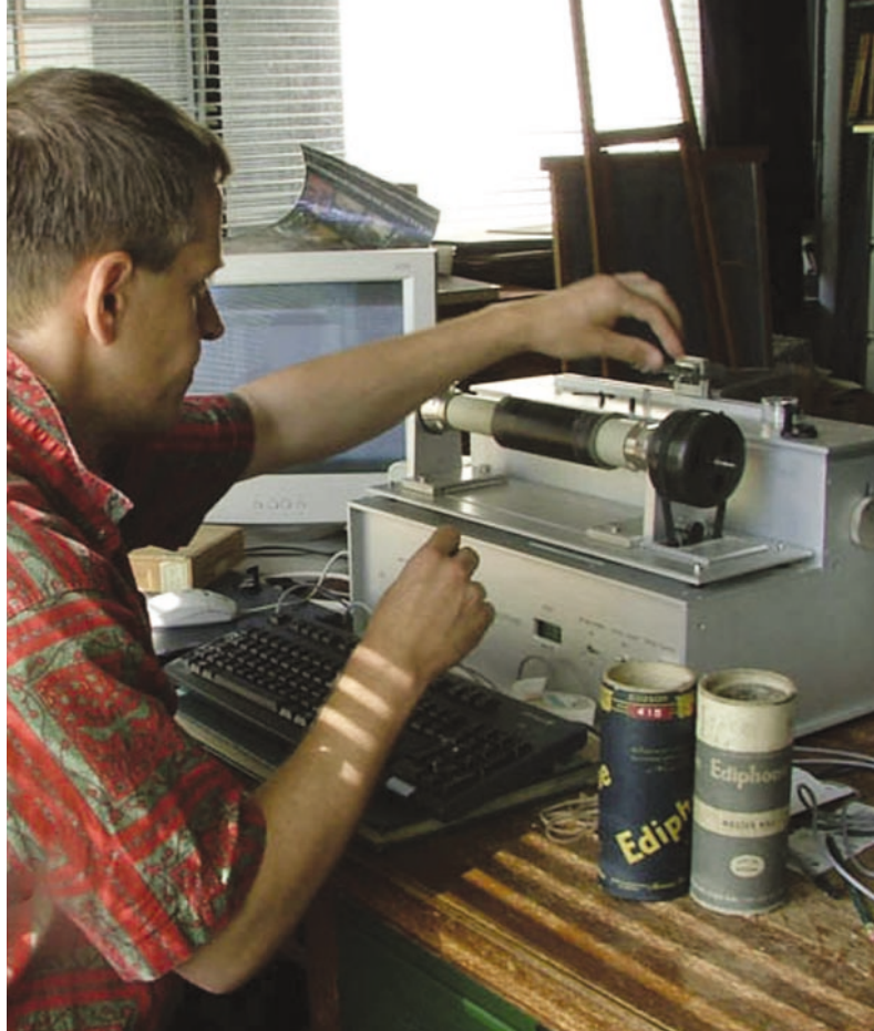
Henri Chamoux, an té a chéadcheap an gléas 'L'Archeophone' ag obair ar dhigitiú na bhfiteáin i Roinn Bhéaloideas Éireann, Lúnasa 2004. Grianghraf le Noreen Barron. [Henri Chamoux, inventor of the 'Archeophone' cylinder reproduction machine, digitising cylinders in the Department of Irish Folklore, August 2004. Photograph by Noreen Barron]
