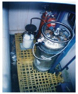
A 27-yr-old postgraduate student was found lying on the floor adjacent to an empty cylinder of liquid nitrogen (150 L) which was connected to an empty Dewarflask (10 L) via a copper infusion tube. No injury was found externally or internally. attributed Death was to nitrogen asphyxiation. How the nitrogen escaped was unclear. The enclosed nature of the area within which the liquid nitrogen was held was deemed to be a contributing factor (see photo).
