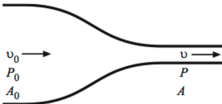
Figure 1: Fluid flow through a pipe of varying diameter
