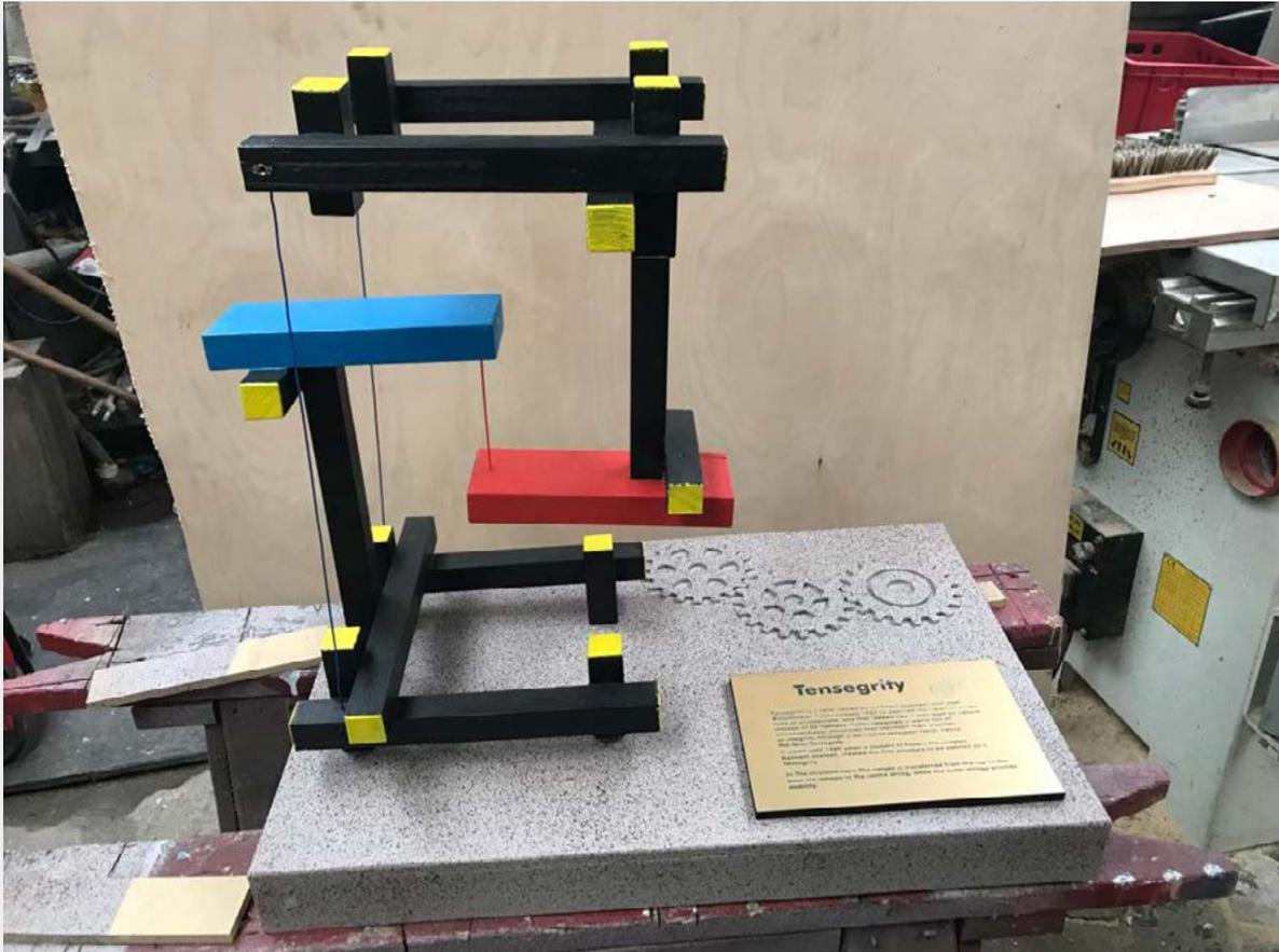
**Figure 1. A tensegrity physical model demonstrated at University for All Symposium May 2022**
