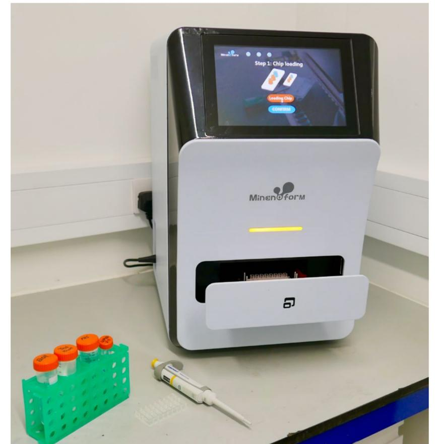
*MiNano-form: a high-throughput nanoparticle formulation system and the microfluidic cartridge developed at UCD.*
